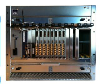
Figure 12: 32 channels ADQ412-MTCA in chassis.
