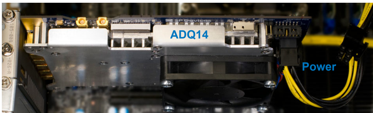
Figure 8: ADQ14 installed in a PC. ADQ7 has the same power supply.
