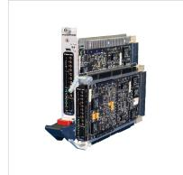
The Jade<sup>®</sup> 52131 is a multichannel, high-speed data converter with multiband DDCs (digital downconverters). It is suitable for connection to HF or IF ports of a communications or radar system. Its built-in data capture feature offers an ideal turnkey solution as well as a platform for developing and deploying custom FPGA-processing IP.
