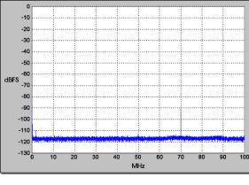
$f_{in}$  Ch2 = 70 MHz,  $f_s$  = 200 MHz, Ch 1 shown
