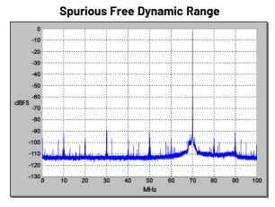
$f_{in}$  = 70 MHz,  $f_s$  = 200 MHz, Internal Clock
