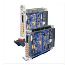
The 52611 is a multichannel, high-speed data converter, suitable for connection to HF or IF ports of a communications or radar system. Its built-in data capture and playback features offer an ideal turnkey solution.
