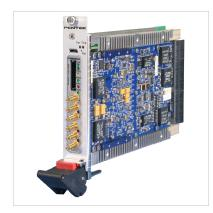
The 52650 is a two-channel, high-speed data converter that is suitable for connection to HF or IF ports of a communications or radar system. Its built-in data capture and playback features offer an ideal turnkey solution.
