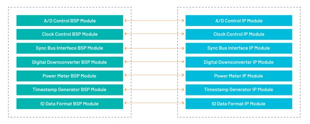
Because all Jade boards are shipped with a full suite of built-in IP functions and numerous software examples, new applications can be developed by building on the provided software examples or built entirely new with the BSP extensive libraries. All BSP libraries are provided as C-language source for full access and code transparency.
