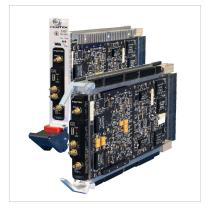
The Jade® 52841 is a high-speed data converter with programmable DDCs (digital downconverters). It is suitable for connection to HF or IF ports of a communications or radar system.
