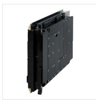
The Quartz<sup>®</sup> 5550 is a high-performance, SOSA aligned 3U OpenVPX board based on the Xilinx Zynq UltraScale+ RFSoC. The RFSoC integrates eight RF class A/D and D/A converters into the Zynq's multiprocessor architecture, creating a multichannel data conversion and processing solution on a single chip. The 5550 brings RFSoC performance to 3U VPX with a complete system on a board.
