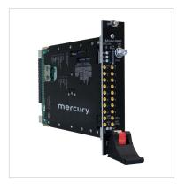
**The Quartz<sup>®</sup> 5950 is a high-performance 3U OpenVPX board based on the Xilinx Zynq UltraScale+ RFSoC FPGA.** The RFSoC integrates eight RF-class A/D and D/A converters into the Zynq's multiprocessor architecture, creating a multichannel data conversion and processing solution on a single chip. The 5950 brings RFSoC performance to 3U VPX with a complete system on a board.
