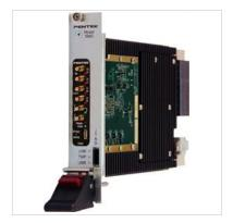
Model 5983 is a member of the Flexor® family of high-performance 3U VPX baseboards with a Xilinx Kintex UltraScale FPGA and an available FMC I/O slot. As an integrated solution, the Model 5983-320 FlexorSet® combines the Model 5983 and the Model 3320 Flexor® FMC as a factory-installed set. The required FPGA IP is installed and the board set is delivered ready for immediate use.
