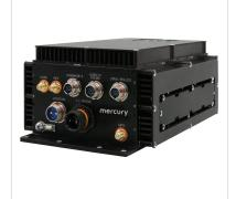
The Quartz® 6350 is a high-performance, small form factor system based on the Xilinx Zynq UltraScale+ RFSoC. The RFSoC integrates eight RF-class A/D and D/A converters into the Zynq's multiprocessor architecture, creating a multichannel data conversion and processing solution on a single chip.
