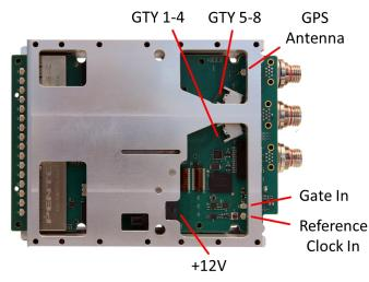
All analog I/O and control and communication interfaces are easily accessible, simplifying connections to other system components.
