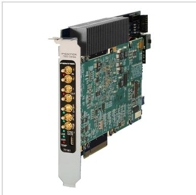
**The Jade® 78141A is a high-speed analog-to-digital and digital-to-analog converter with programmable DDCs (digital downconverters) and DUCs (digital upconverters).** It is suitable for connection to HF or IF ports of a communications or radar system.
