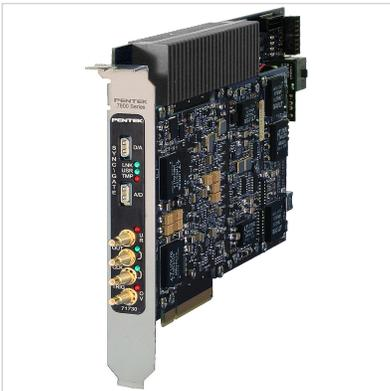
**The 78730 is a high-speed data converter, suitable for connection to HF or IF ports of a communications or radar system.** Its built-in data capture and playback features offer an ideal turnkey solution as well as a platform for developing and deploying custom FPGA processing IP.
