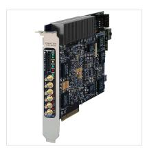
The 78751 is a high-speed data converter with a programmable digital downconverter, suitable for connection to HF or IF ports of a communications or radar system. Its built-in data capture and playback features offer an ideal turnkey solution as well as a platform for developing and deploying custom FPGA processing IP.
