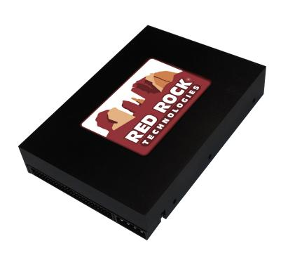
THE 3.5" SCSI 50-PIN NARROW SOLID STATE DRIVE (SSD) uses a proprietary FPGA-based design that provides a long-term solution for replacement of obsolete SCSI drives.
