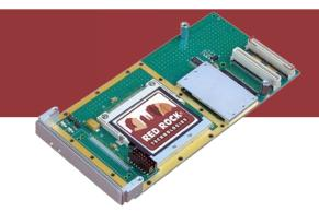
The Conduction Cooled PMC Compact Flash (CF) module is a PMC mezzanine storage module with a FPGA based PC/ATA/IDE controller that supports on fixed compact flash. Ruggedized for extreme temperature, shock and vibration environments. Provides boot drive and/or disk storage for conduction cooled VME, VPX, CPCi and ATCA single board computers (SBCs) with a PMC slot.
