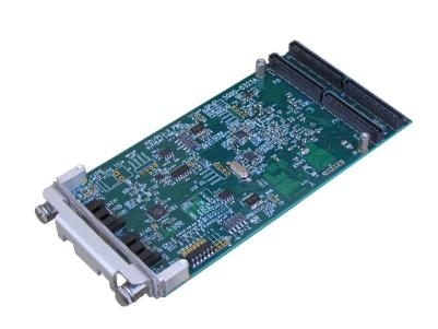
THE PMC SATA CONTROLLER is a PMC Mezzanine card with a dual-channel 64-bit PCI/PCI-X SATA 3 controller with 2 SATA connectors via front panel.
