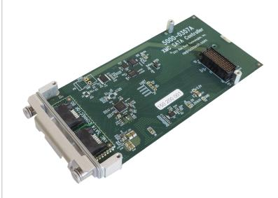
THE XMC SATA CONTROLLER is an XMC Mezzanine card with a dual-channel PCIe Gen 2x2 SATA 3 controller with 2 SATA connectors via front panel.
