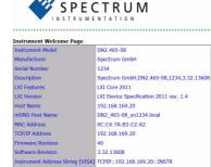
The integrated webserver follows the LXI standard and gathers information on the product, set up of the Ethernet configuration and current status. It also allows the setting of a configuration password, access to documentation and updating of the complete instrument firmware, including the embedded remote server and the webserver
