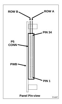
The 68-pin DSUB (user I/O interface) connector (PLUG) is mounted at the front edge of the board. The part number is P50E-068DDP-SRI-TG, manufacturer, Robinson Nugent. The mating part number is 3M Corporation P50-068-DDS-EA, Backshell: P50-068-STR-BSK
