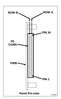
The 68-pin DSUB (user I/O interface) connector (PLUG) is mounted at the front edge of the board. The part number is P50E-068DDP-SRI-TG, manufacturer, Robinson Nugent. The mating part number is 3M Corporation P50-068-DDS-EA connector with P50-068-STR-BSK backshell Contact GSC for factory built cables of any desired length. See Table above for pin-out.
