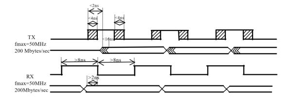
Note: Data is transmitted on the rising edge of the Transmit clock and received on the negative edge of the receive clock.
