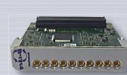
ACQ480FMC (80MHz 14bit 8ch A/D)
