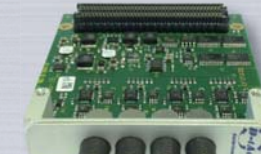
AO420FMC (2MHz 18bit 4ch A/D)
