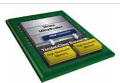
図34. Xilinx製 Virtex UltraScale+のHBM Gen2
